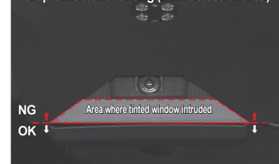
Part prohibited for tinting (FCM detection area)
