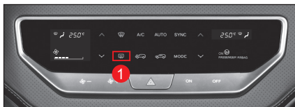
Rear window heater
