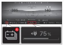
Indicates the state of charge of the high-voltage battery (drive battery).
