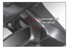
The rain sensor is integrated with the auto light sensor.
