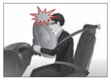
If the air bag control module detects the impact during an accident, it transmits the signal to deploy the air bag. This signal triggers the explosion of the powder, which is included in the air bag module, and the air bag deploys in a very short time to protect the occupants. When the air bag inflates, there will be heavy noise, glare and smoke. You could suffer secondary injuries caused by inflated air bag such as an abrasion, a bruise, a burn or injury by broken glasses.
