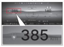
DTE shows the approximate distance your vehicle can travel before running out of power. The DTE value is calculated based on the current SoC of the HV battery, the driving mode (SPORT, ECO, ECO+), and the accumulated data on the driver's driving pattern.
