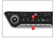
To use the heating system, press the heating mode switch (1). Then the operation indicator (2) shall be turned on and the heater temperature can be adjusted according to the setting temperature.
