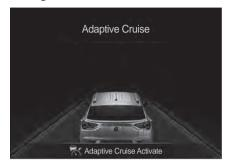
When detecting the lanes according to the vehicle condition, the detected lane is displayed in white and alarm can be issued at the detected lane. Depending on the operating system, the front vehicle is displayed.
