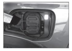
3 Check if there is any dust or fluid on and around the charge port and install it.
