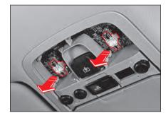
After replacing it, install the cover again.
