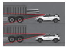
Caution should be taken that a tall vehicle or a vehicle with cargo sticking out the back of the vehicle may cause a dangerous situation.
