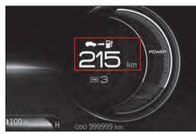
DTE shows the approximate distance your vehicle can travel before running out of power. The DTE value is calculated based on the current SoC of the HV battery, the driving mode (SPORT, ECO. ECO+), and the accumulated data on the driver's driving pattern.
