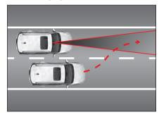
When a vehicle on the next lane changes the lane to the same lane, the vehicle may not be detected until it enters the detection range of the Front Camera Module (FCM).
