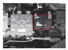
If the low voltage battery charge warning lamp (-+) illuminates while driving, there is a fault in the charging system of the vehicle including the low voltage (12 V) battery. In this case, immediately have the vehicle checked and serviced at a KG Mobility Dealer or KG Mobility Authorized Service Center.
