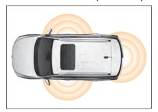
When you move a certain distance away from the vehicle while carrying the smart key, all doors and the tailgate are locked automatically.
