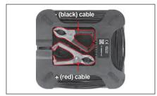
Connect the + (red) (1) cable of the service kit to the vehicle battery and then connect the - (black) (2) cable.
