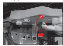
3 Check the charging connector is released before removing it.
