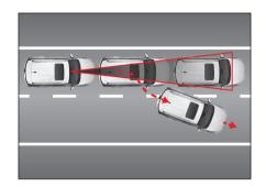
Caution should be taken that if there is a vehicle stopped in front of the vehicle ahead and the vehicle ahead moves out of the lane while your vehicle has been decelerated due to the AEBS operation, the vehicle stopped at the front is not selected as the control target, causing a collision risk
