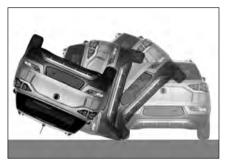
If the vehicle turns over or rolls over, the occupant cannot be protected fully by the air bag alone. In such case, the air bag may not inflate.
