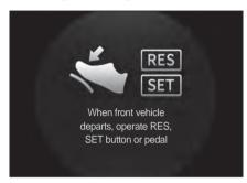
When the intelligent cruise control is operating, in congested areas, drive the vehicle while maintaining the distance to the front vehicle constant. Depress the accelerator pedal or push up the speed selector lever toward RES+ briefly or lower it toward SET- briefly to restart the vehicle 3 seconds after since the vehicle stops due to the front stationary vehicle.
