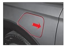
5 Pull the charge port door in the direction of the arrow to open it.
