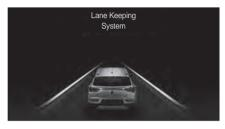
When both lane lines are detected while the vehicle is being driven at 40 km/h or more, both the lane markers on the display turns green.
