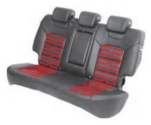
Every time the heating button is pressed, the warmer is operated in the order of OFF → Level 2 → Level 1 → OFF.
