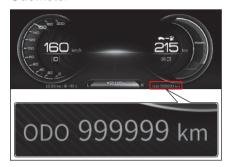
The total mileage of the vehicle is displayed in kilometers. The maximum mileage to be displayed is 999999 km.
