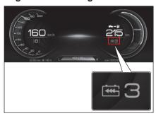
The number shown below the DTE during regenerative braking indicates the regenerative braking level currently engaged.
