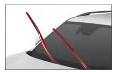
Press the wiper blade retainer (1) and pull the wiper blade out in the arrow direction (2).
