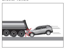
Generally, most drivers apply a sudden brake when an accident occurs, so the front part of the vehicle becomes lower. Therefore, the vehicle often moves beneath the opposing vehicle in the event of an accident against a tall vehicle such as a bus or a truck. In such case, the air bag may not inflate.
