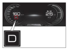
This indicator shows the current position of the electronic shift lever (P, R, N, D).
