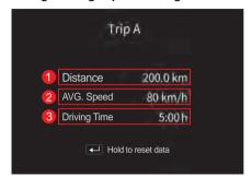
The distance that the vehicle traveled (km), average speed (km/h) and driving time (hh:mm) are displayed.
