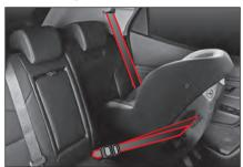
Secure the child restraint with a seat belt as shown in the figure.
