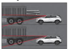
Your attention is always required while driving behind a vehicle carrying cargo longer than the cargo bed or with high ground clearance because the AEBS may not work properly.
