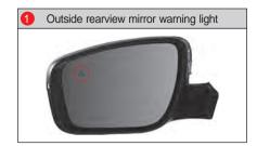
When the outside rearview mirror warning light blinks twice with the START/STOP switch in the ON status or while the vehicle is running, it indicates that the rear and side warning system is operating normally.
