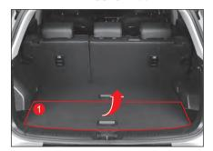
1 Lift out the luggage compartment board (1) in the direction of the arrow.
