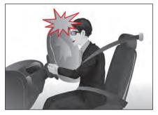
If the air bag control module detects the impact during an accident, it transmits the signal to deploy the air bag. This signal triggers the explosion of the powder, which is included in the air bag module, and the air bag deploys in a very short time to protect the occupants. When the air bag inflates, there will be heavy noise, glare and smoke. You could suffer secondary injuries caused by inflated air bag such as an abrasion, a bruise, a burn or injury by broken glasses.
