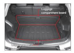
The luggage compartment board can be stored as shown in the picture and the luggage compartment cover is located at the bottom of it.
