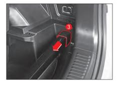
3 Pull the left / right end (3) of the luggage compartment upper cover inward and fix it in the groove. The other side is also performed in the same way.
