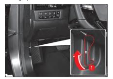
2 Lift the motor room hood slightly to pull the motor room hood latch lever (2) up and lift up the motor room hood completely.
