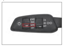
2 Push the Light switch in the direction of instrument cluster and release it.
