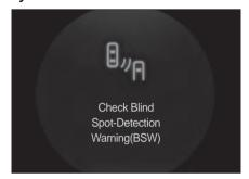
When the rear and side warning system is abnormal, a warning message is displayed on the display of the instrument cluster.
