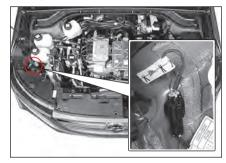
Cut the safety interlock connector to cut off the battery high voltage in an emergency.
