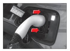
Align the charging connector to the charge port and insert completely.
