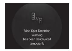
If the sensor cannot detect the rear and both side areas of the vehicle normally with the rear and side warning system activated, the message is displayed on the display of the instrument cluster.
