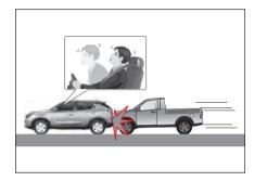
In the event of a rear end collision by another vehicle, the body of the occupants move backwards, so the air bag cannot provide enough protection even if it inflates. In such case, the air bag may not inflate.
