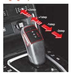
The electronic shift lever can be moved at + 2 step and - 2 step, after which it is always aligned to the central position.
