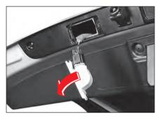
4 Remove the license plate from the socket and replace it with new one with right specifications.
