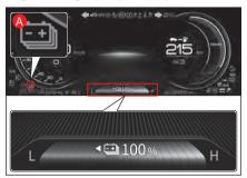
This gauge consists of 20 short bars and indicates the state of charge (SoC) of the HV battery (drive battery).
