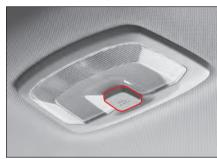
Press the center room lamp switch to turn the lamp on and press it again to turn it off.
