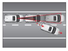
If the front vehicle leaves the lane due to lane change, etc., be careful that there is a risk of collision because the system can not detect another vehicle ahead.
