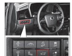
Press and hold the Tailgate button on the driver seat.
