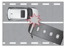
Since the impact of a collision in the diagonal direction is weaker than the impact of a collision in the front or side direction, the air bag may not inflate.
