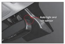
The auto light sensor is integrated with the rain sensor.
