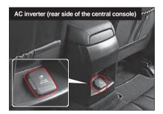
The AC inverter is a convenient device that converts the DC 12 V electricity provided by the vehicle into the 220V (200W) [115V (150W)] that is the electricity for homes, allowing you to connect and use a simple electrical appliance such as the laptop computer, smartphone, mobile TV, lighting equipment, battery charger, etc.
