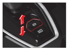
Operate the EPB (Electroic Parking Brake) switch and check the operating sound and operation status.
