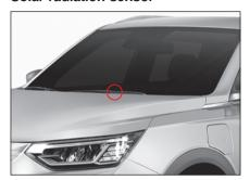
The solar radiation sensor is mounted on the top of the instrument panel (IP). It detects solar radiation and automatically adjusts the vehicle interior temperature according to the amount of solar radiation, when the user selects "AUTO" on the heater and air conditioner controller.
