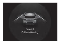
If the distance to the front vehicle is so close that a collision can occur or the front vehicle disappears from the front view due to lane change, etc. while the intelligent cruise control is activated, the message is displayed on the instrument cluster.
