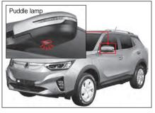
The welcome light is the function that operates the puddle lamp and the door handle lamp in order to increase safety and visibility at night.
