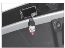
Once replacement is completed, assemble the lamp in reverse order of removal.
