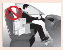
Before driving the vehicle, clean up the area where the brake pedal or the accelerator pedal is operated. If an empty can or an article is present below the pedal, it may obstruct the pedal operation, causing an accident. Be sure to check before driving the vehicle.
