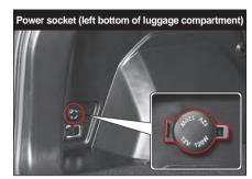
The power socket (12 V, 120 W) is provided in the vehicle to enable the use of a separate electrical device.
