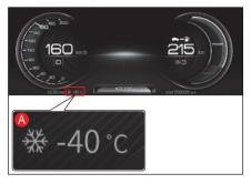
This Indicator displays the current ambient temperature.
