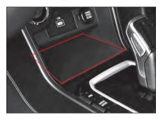
The front storage is provided near the SBW (shift by wire). Use it for storing a small article.
