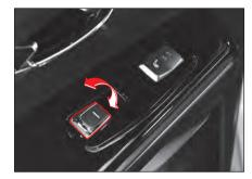
The window only works while pressing or pulling the rear seat window button.
