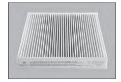
3 Replace with new one. Make sure that the "AIR FLOW" arrow faces toward the driver seat.
