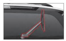
With the wiper blade lifted to its side, remove it by pulling it in the arrow direction.
