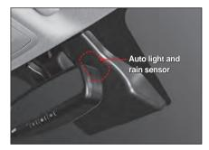
The rain sensor is integrated with the auto light sensor.
