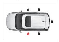
Pressing the Door unlock button (2) again with the driver seat door unlocked unlocks all doors and the tailgate.
