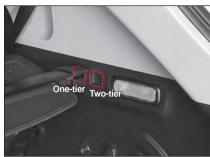
The luggage upper cover can be fixed at the position of one-tier or two-tier according to the angle adjustment level of the rear seat backrest.
