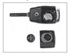
3 Return the cover from the back of the smart key back to its original position.
