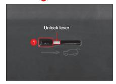
3 Press the mechanical key in the direction of the arrow. It unlocks the tailgate.
