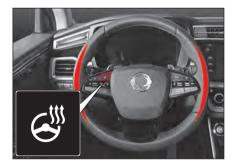
· To activate the steering wheel heater, press the steering wheel heater switch while the vehicle is running.
