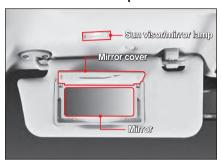
When you pull the sun visor down and open the mirror cover, the lamp turns on.
