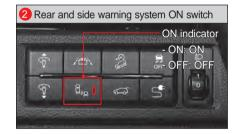
When you turn off the vehicle with the rear and side warning system deactivated and set the START/STOP switch to the ON status, the system turns on without returning to the previous status.
