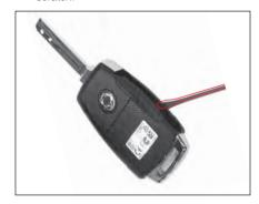
Insert the battery with the positive (+) terminal facing up and the negative (-) terminal facing down.
