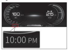
This clock displays the current time as set in the audio system in digital format.
