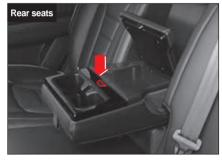
Articles used by occupants can be stored on the console at the front seats and the rear seats. conveniently.
