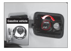
7 Hang the fuel inlet cap on the holder mounted inside the fuel inlet cover.
