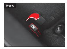
For the diesel-powered vehicles, press the center edge of the fuel filler door in the direction of the arrow.
