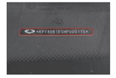
The VIN is stamped on top of the instrument panel.
