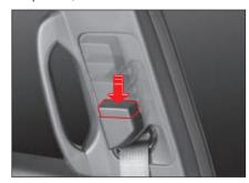
Release it at the desired position. The seat belt holder is secured.
