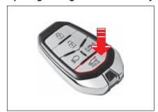
Press and hold the Tailgate button on the smart key.
