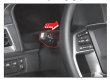
The high beam and the low beam turn on at the same time while pulling the Light switch in the driver's direction.
