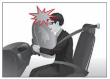
If the air bag control module detects the impact during an accident, it transmits the signal to deploy the air bag. This signal triggers the explosion of the powder, which is included in the air bag module, and the air bag deploys in a very short time to protect the occupants. When the air bag inflates, there will be heavy noise, glare and smoke. You could suffer secondary injuries caused by inflated air bag such as an abrasion, a bruise, a burn or injury by broken classes.
