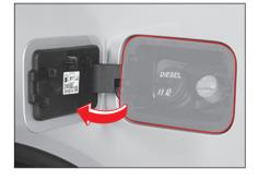
6 Open the fuel inlet cap by turning it counterclockwise.
