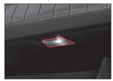
When you open the glove box, the lamp turns on, and when you close the glove box, the lamp turns off.
