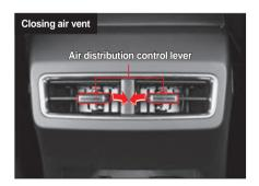
You can close the air vent by pushing the air distribution control lever all the way in the direction of the arrow.
