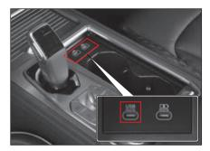
A USB storage device, an external music and video player such as iPod/iPhone/iPad, an MP3 player can be connected to the vehicle through the USB port (type C).
