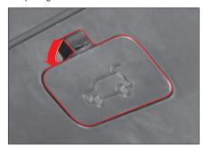
2 Push the unlock lever in the arrow direction. The tailgate will be unlocked.
