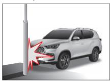
In the event of a collision with a narrow object such as a street light, utility pole or tree, the degree of impact applied to the sensor may not be enough, so the air bag may not inflate.
