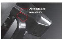
The rain sensor is integrated with the auto light sensor.
