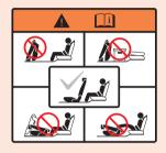
· Do not drive the vehicle or load any cargo while the rear 1st row seat is in the vertical position.
