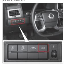
Press and hold the Tailgate button on the driver seat.
