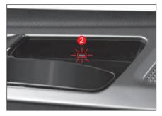
It turns on when the tail light is activated. It softly lights up the front door handle.
