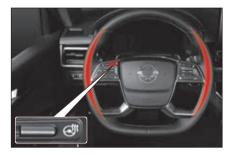
To activate the steering wheel heater, press the steering wheel heater switch while the engine is running.
