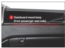
Mood lamps are always activated when any door is open, the ignition is turned on, or switch is turned on, as long as they are set to on.
