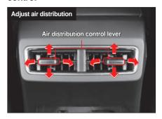
You can adjust air distribution by moving the air distribution control lever at the vent up and down and left and right.
