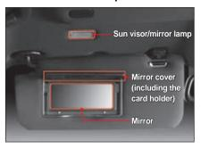
When you pull the sun visor down and open the mirror cover, the lamp turns on.
